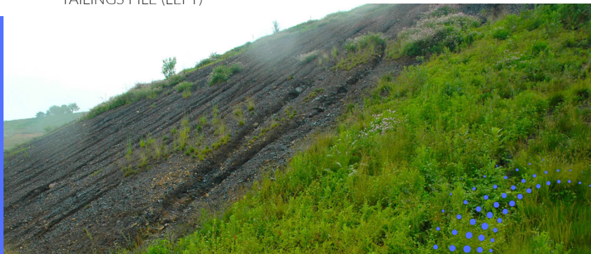
COMPARISON OF AN AREA WHERE THEY USED THE REACTIVE CAP TECHNOLOGY (RIGHT) VERSUS APPLYING SEED MIX ON A TAILINGS PILE (LEFT)
